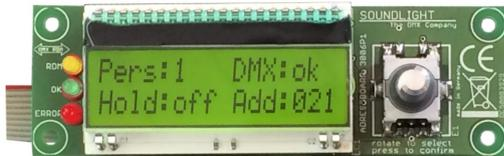
Start address board with LCD display and rotary encoder to set the DMX start address. Address is retained in non-volatile onboard memory.
